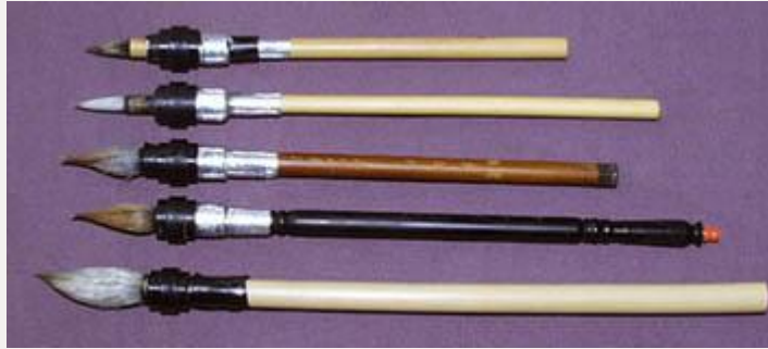
Oriental brushes with ferules adapted to fit the pen plotter.
